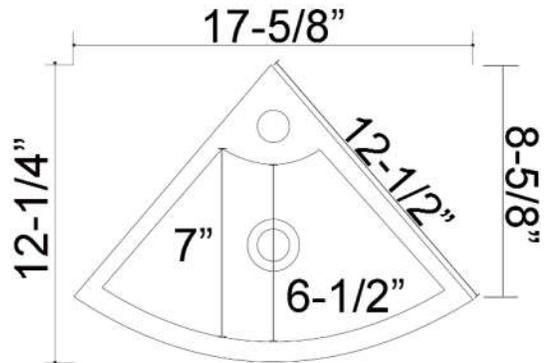
Dimensions of fixture are nominal and may vary within the range of tolerances established by ANSI Standard A112.19.2.2018. Dimensions and specifications subject to change without notice.
