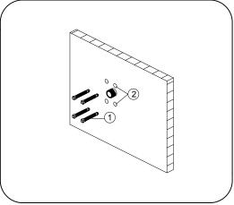
4.Insert anchors (1) into holes (2) and tap flush with
